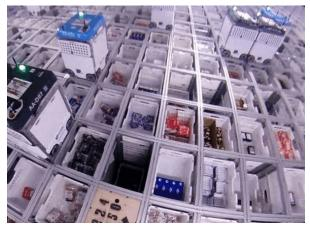
along a matrix of tracks with tote bins or boxes below, so a robot is able to drop something in the box just by parking over it, to ultimately be delivered to a customer. You see five robots in the picture, two with blue tops and three with black. Each has two sets of four wheels, where the robot can raise one set and lower the other to change directions, allowing it to easily go back and forth or up and down the track rows at will.
